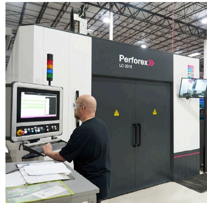
The Perforex LC laser centre is ideal for the automated mechanical modification of stainless steel and sheet steel enclosures.
