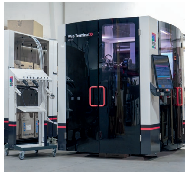
Usemco uses the Rittal Wire Terminal WT C for fully automated wire processing.
