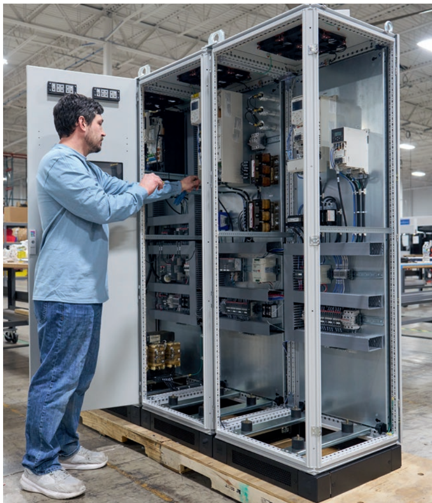
The flexibility of Rittal enclosures makes them very popular in production departments. The rear panel, side panels and roof are all easy to remove.
